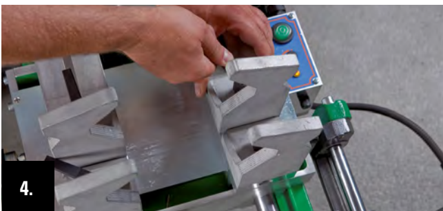
4. For pipe fixing, push the back pair of clamping jaws at the front pair of clamping jaws and fix it by tightening of the fixing screws.
