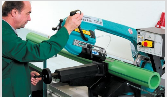
Before welding, pipes are cut into the required lengths
