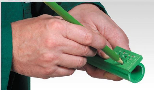
Marking of the welding depth
