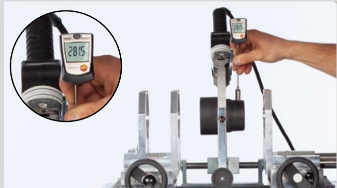
Measurement of temperature at the aquatherm welding machine
