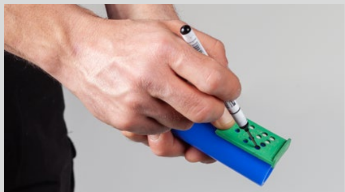
Marking of the welding depth
