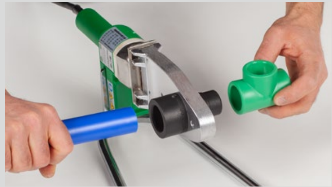
Heating-up of pipe and fitting
