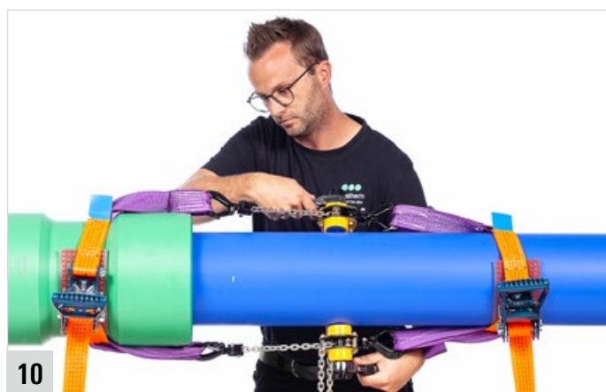
Pull the push-fit fitting onto the pipe end up to the marked insertion depth.
