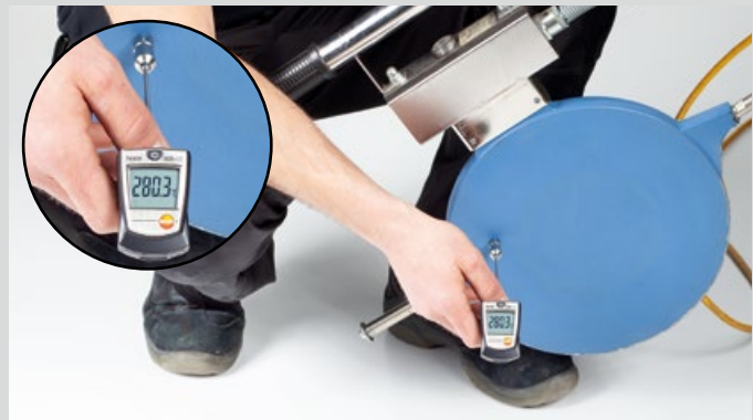
Measurement of temperature at the aquatherm butt-welding machine
