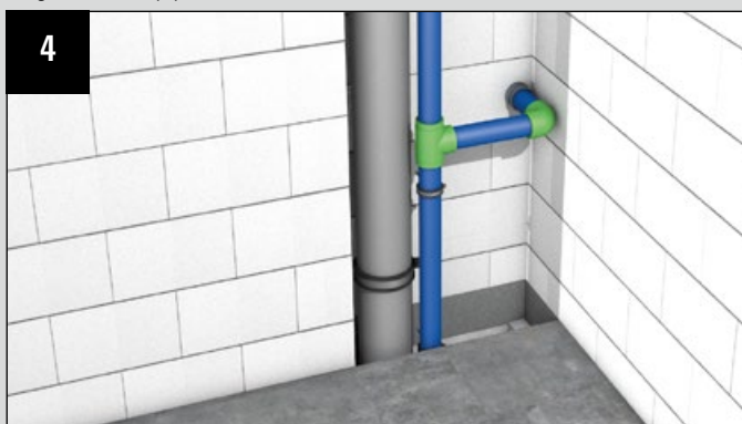
Installation of a spring leg
